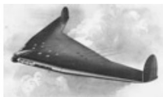
An artists impression of the Armstrong Whitworth design for a six-engined Flying Wing with accommodation for passengers within the central wing area.
